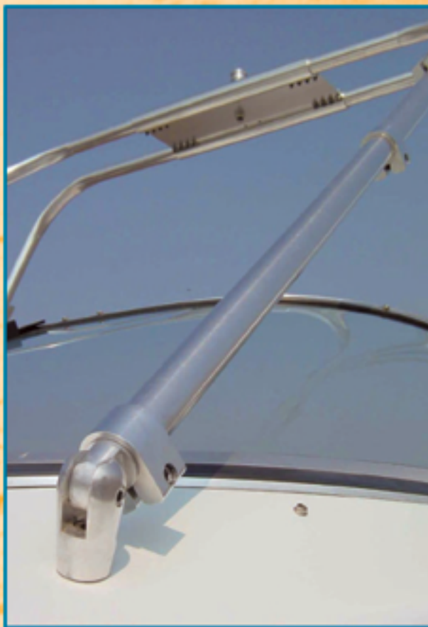
Universal foot assembly facilitates mounting to virtually any boat surface
