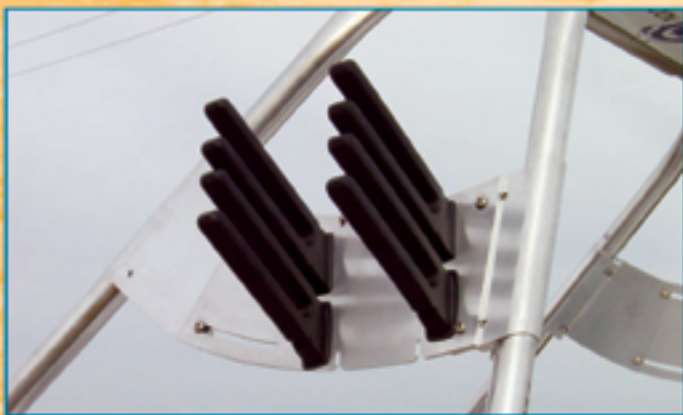
Board racks covered with replaceable vinyl sleeves to prevent damage to wake board and skis
